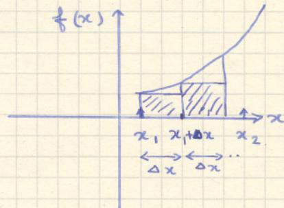
The interval  $\underline{x_2 - x_1}$  is divided into a number of smaller intervals ( $\Delta x$ ). When  $\Delta x$  is small the shaded rectangles will have area approximately equal to the area between the  $x$  axis and the function between  $x$  and  $x + \Delta x$  (for the left most segment in the figure). This is equal to  $f(x_1) \Delta x$
